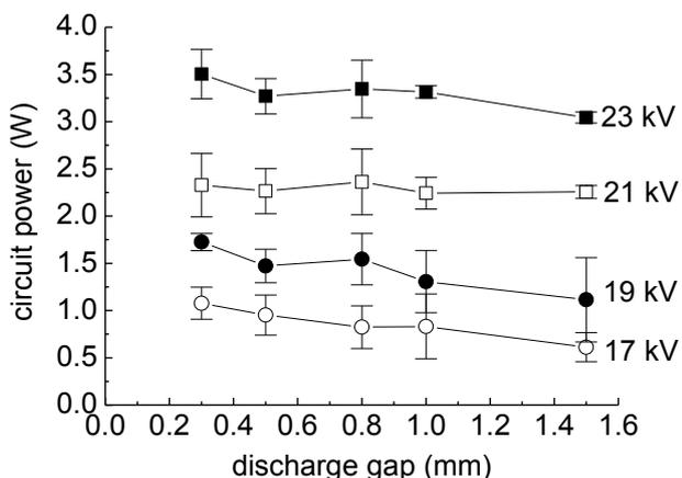
**Fig. 3.** Mean power (see Eq. 1) delivered to the system (without specimen) as a function of the discharge gap, with the applied voltage (peak-to-peak) as parameter. Mean values and standard deviations from three experimental series are given.
