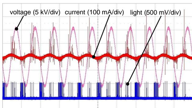
**Fig. 2.** Typical voltage, current and light waveforms over ten periods of the applied voltage (1 mm discharge gap, 23 kV peak-to-peak, 100  $\mu$ s/div, without specimen).
