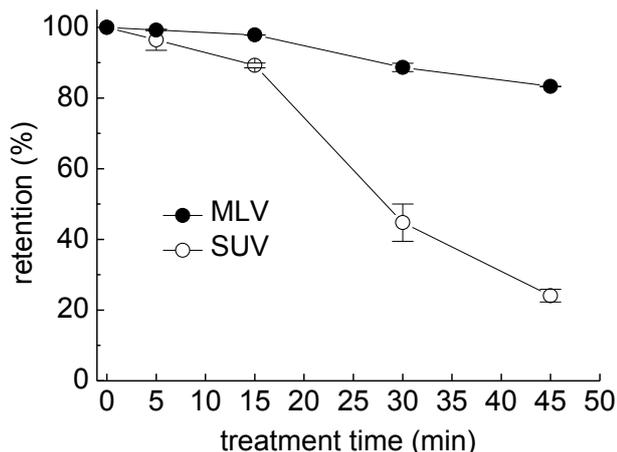
**Fig. 6.** Effect of the FE-DBD reactor on SUV and MLV liposomes treated for various times (19 kV peak-to-peak,  $\sim 1$  mm gap between the dielectric and aqueous solution surfaces). Mean values and standard deviations from two experimental series are given.
