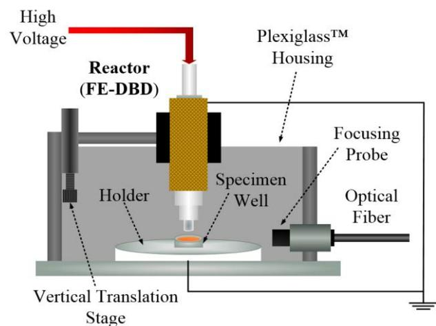
**Fig. 1.** Schematic diagram of the FE-DBD reactor installed in protective housing for liposome treatment. The holder and the specimen well are both grounded.
