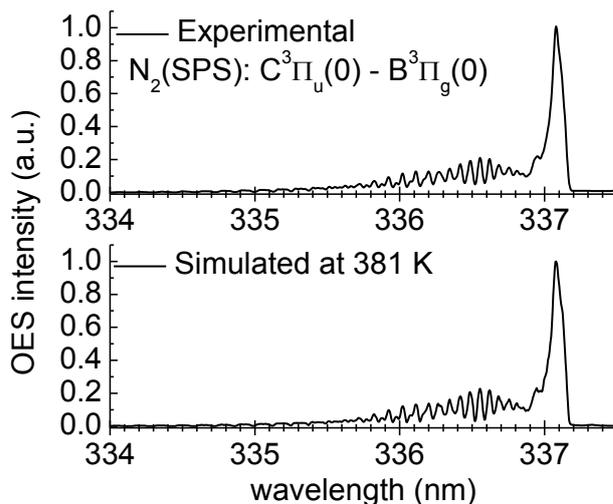
**Fig. 5.** Typical experimental and simulated optical emission spectra (resolution 0.005 nm) of the rotational distribution of the  $N_2$ (SPS) band corresponding to the transition  $C^3\Pi_u(0) - B^3\Pi_g(0)$  (1 mm discharge gap, 23 kV peak-to-peak, without specimen). For 17-23 kV peak-to-peak the gas temperature does not change significantly.
