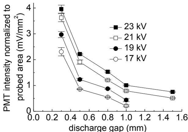
**Fig. 4.** Normalized mean values of the optical emission intensity integrated over time (PMT) and space (entire discharge gap), as a function of the gap distance, with the applied voltage (peak-to-peak) as parameter. Mean values and standard deviations from three experimental series are given.
