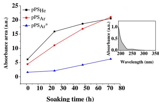
Fig. 5: Water stability of pPS<sub>He</sub> and pPS<sub>Ar</sub> films. Insert: UV spectrum of water in which the pPS<sub>He</sub> was soaked for 72 h.
