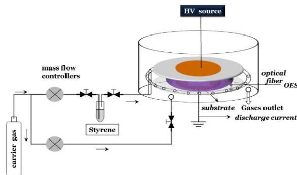
Fig. 1. Schematic representation of the plasma polymerization system.
