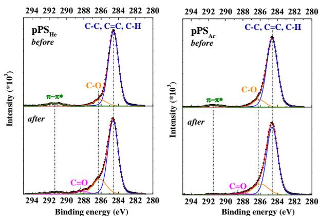
Fig. 3: High-resolution XPS C1s spectra of pPS<sub>He</sub> and pPS<sub>Ar</sub> before and after 72 h of immersion in water.
