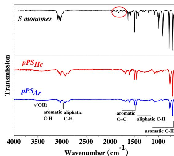
Fig. 2. FTIR spectra of monomer S, pPS<sub>He</sub> and pPS<sub>Ar</sub> deposited onto NaCl plates.
