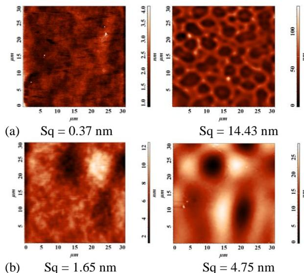
Fig. 6: AFM topographic images  $30 \times 30 \mu\text{m}^2$  of the (a) pPS<sub>He</sub> and (b) pPS<sub>Ar</sub> films before and after immersion in distilled water for 24 h.
