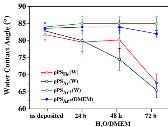
Fig. 4: Water contact angles measured as a function of immersion time in water (W) and cell culture medium (DMEM). Error bar shows a standard deviation of 10 drops for one sample.
