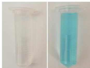
Fig. 3. MB samples (MB mixed with distilled water treated for 50 minutes – left; control – right) two days after preparation.
