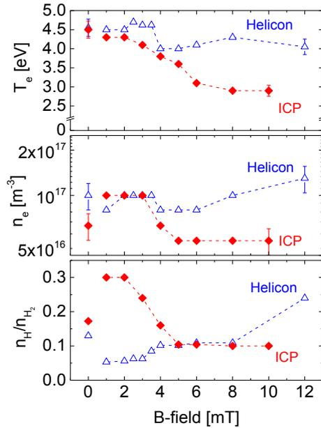
Figure 3: Electron temperature, electron density and density ratio of atomic to molecular hydrogen with varying magnetic field for both ICP- and Helicon-setup.
