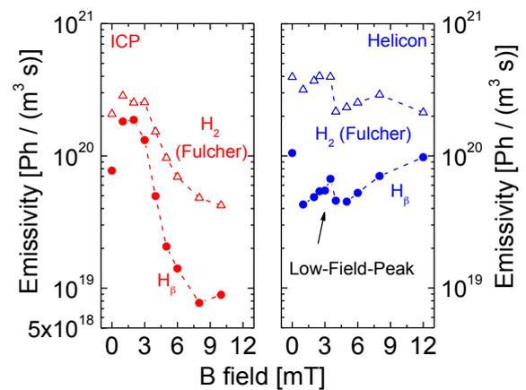
Figure 2: Emissivity of the atomic H $\beta$ -line and the molecular Fulcher radiation at varying magnetic field for the ICP- and the Helicon-configuration as measured with axial LOS.
