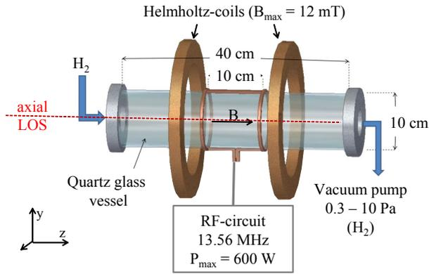
Figure 1: Sketch of the experimental setup. The application of the Nagoya-Type-III helicon antenna is shown exemplarily. Alternatively, a helical ICP-coil (5 windings) can be applied.
