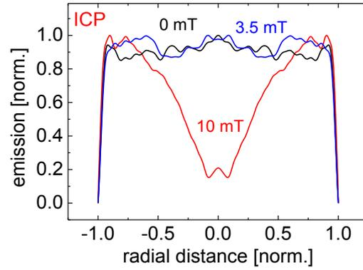
Figure 4: Radial emission profiles of the atomic  $H_\beta$ -line for the ICP-configuration determined via Abel-inversion at different magnetic field strengths.
