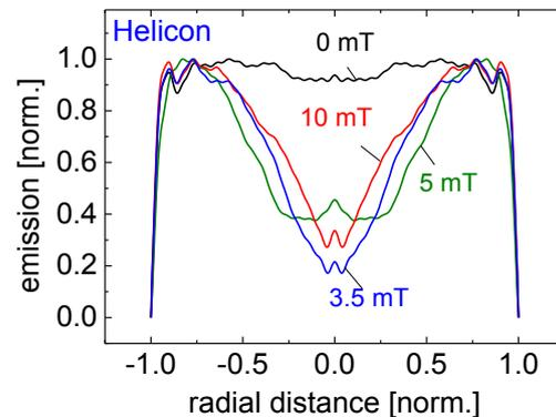
Figure 5: Radial emission profiles of the atomic  $H_\beta$ -line for the Helicon-configuration determined via Abel-inversion at different magnetic field strengths.
