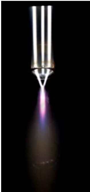
Fig. 1: Picture of the jet behaviour with association of filaments and afterglow generation.
