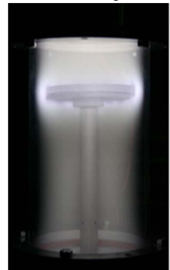
Figure 1. Image of the low pressure plasma device during PE beads treatment
