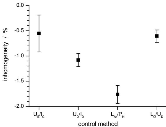
**Fig. 5: Level of inhomogeneity obtained for deposition series using different control methods.**
