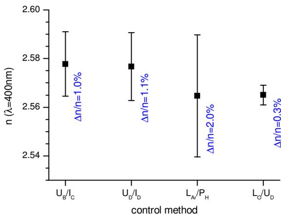
**Fig. 4: Resulting absolute value and variation of refractive index obtained for deposition series using different control methods.**
