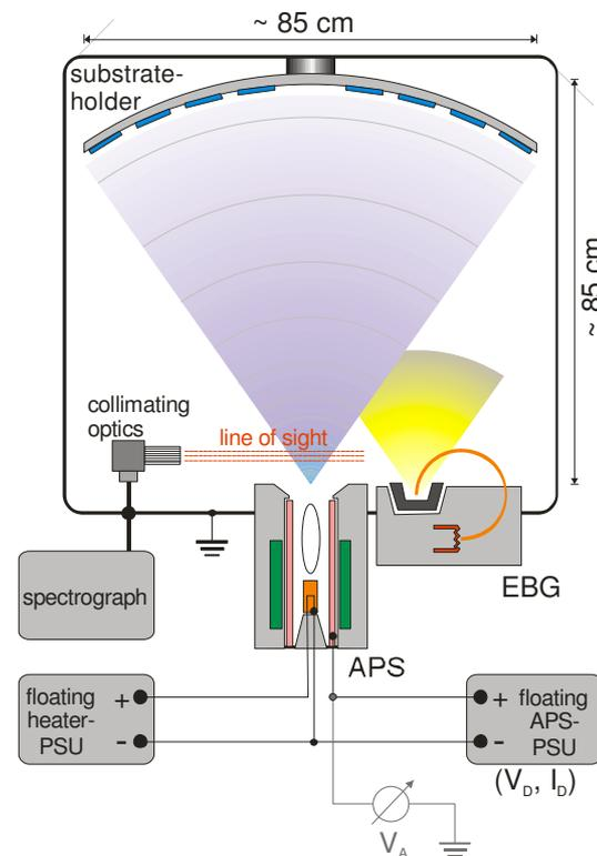
Fig. 1: Scheme of the box coater equipped with plasma source (APS), electron beam evaporator (EBG) and diagnostics (OES).
