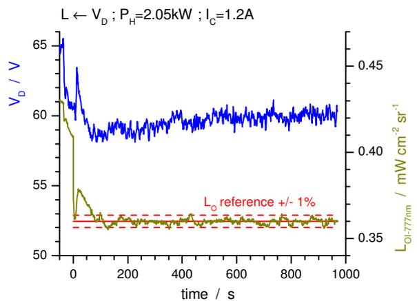
Fig. 3: Time traces of discharge voltage and radiance reference signal in  $L_O/P_H$  controlled deposition phase.
