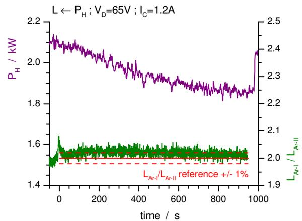
Fig. 2: Time traces of cathode heating power and radiance reference signal in  $L_{ArI}/P_H$  controlled deposition phase.
