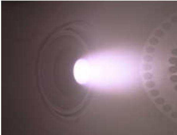
Fig. 2. The nitrogen ions beam emitted from the hollow anode
