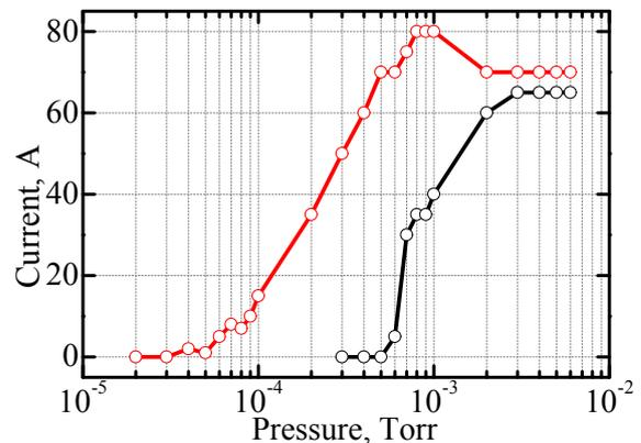
Fig. 3. Discharge current between hollow anode and chamber: black curve – without connection of ring electrode 8 to structure of hollow anode; red curve – the ring electrode 8 is connected to hollow anode
