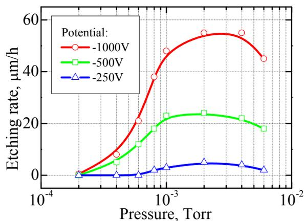
Fig. 5. The pressure dependence of etching rate of stainless steel sample by argon ions ejected from hollow anode. The surface of sample is oriented at the angle of 60 degrees to the direction of ion flux
