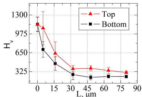
Fig. 4. Microhardness distribution along a depth of Ti plate after nitriding at 850 °C in tangential to the surface ion flux;  $P=1 \cdot 10^{-3}$  Torr; Top - side turned to stream of ions; Bottom - back side, attached to the holder; time of nitriding is 20 min
