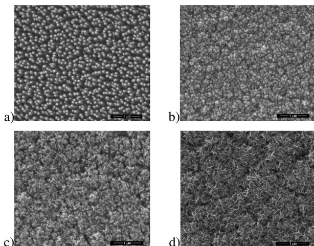
Figure 5. Top-view SEM images of the carbonic material deposited at different substrate temperatures: a) 200°C; b) 400°C; c) 500°C; d) 700°C. Length of scale bar is 1 μm
