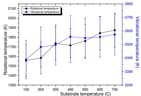
Figure 4: Rotational and vibrational temperatures as function of substrate temperature
