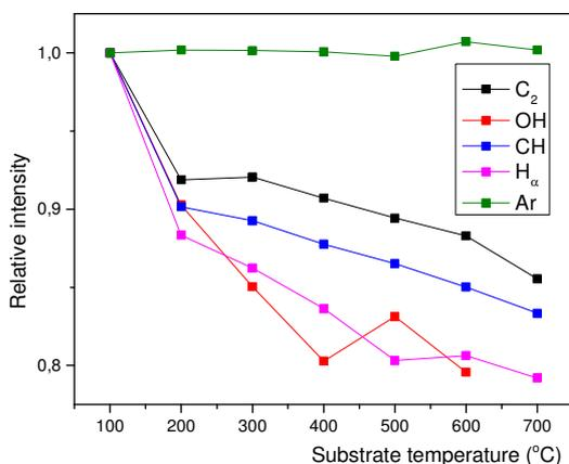
Figure 3: Dependence of the relative intensities of emissive species as function of substrate temperature
