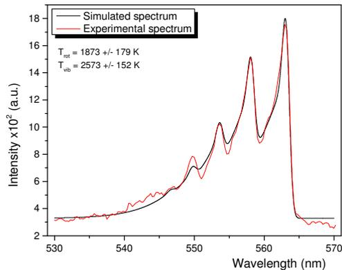
Figure 2: Temperature (rotational and vibrational) determination from  $C_2$  bands (swan system, degraded to violet)
