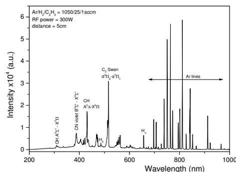
Figure 1: Typical emission spectrum recorded at substrate level
