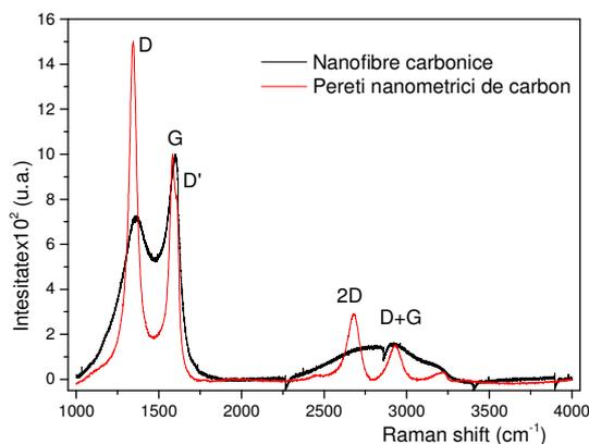
Figure 6: Raman spectra of carbonic structures like CNF and CNW obtained at variation of substrate temperature
