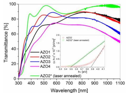
Figure 2. UV-vis spectra of SPLD AZO samples; the inset represents the Tauc plots for BG determination for as deposited (AZO2) and laser annealed (AZO2\*) samples.
