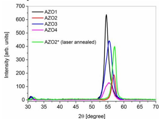
Figure 1. XRD diffractograms of obtained SPLD AZO samples.
