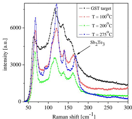
Figure 4. The Raman spectra of GST-124 target and deposited films on Si substrate at various temperatures.
