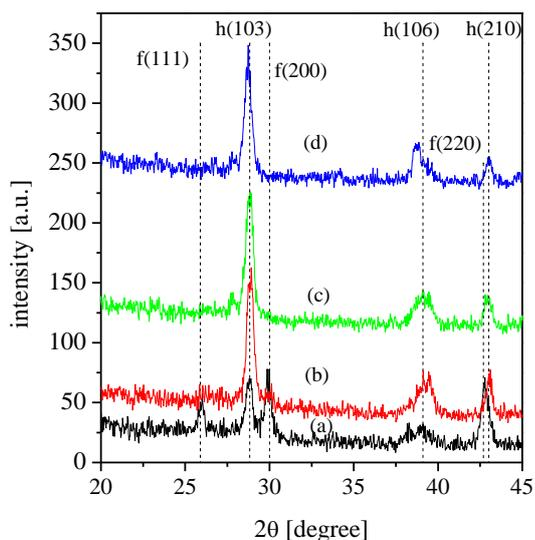
Figure 2. The X-ray pattern of GST-124 film, a) annealed temperature,  $T = 200^{\circ}\text{C}$ , b)  $T = 225^{\circ}\text{C}$ , c)  $T = 275^{\circ}\text{C}$  and d)  $T = 375^{\circ}\text{C}$ .
