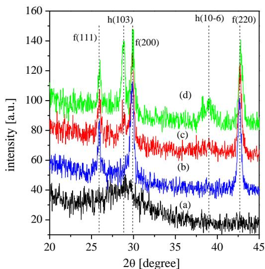
Figure 1. The X-ray pattern of GST-124 film, a) annealing temperature, T=150°C, b) T = 175°C, c) T = 175°C and d) T = 200°C.
