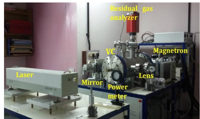
Fig. 1. Digital picture of the laser ablation setup in the background microwave plasma.
