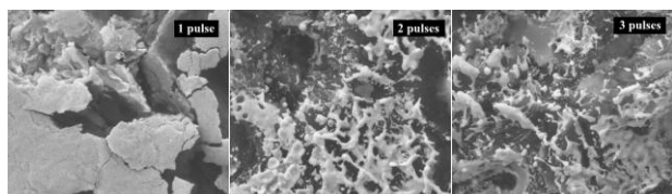
Fig. 3 SEM details of central irradiated area surface for the C/W/graphite structure.
