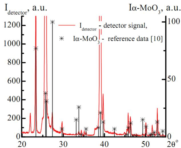
Fig. 7. XRD diagrams for  $\text{MoO}_3$  crystals
