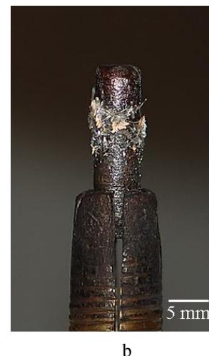
Fig. 1. Experimental scheme of electric arc plasma source (a) and general view of anode with deposited MoO<sub>3</sub> crystals (b)
