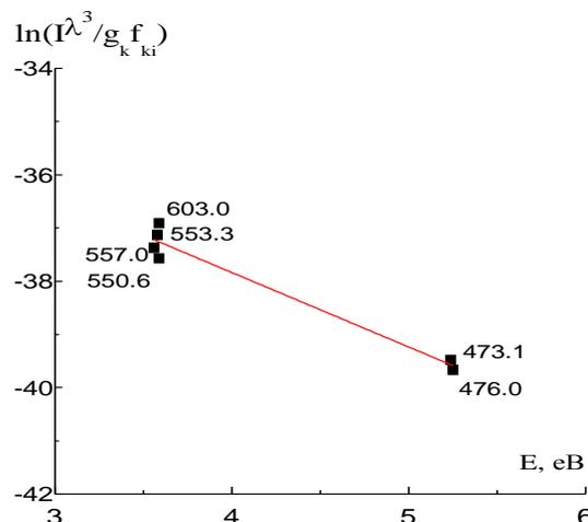
Fig.4. Boltzmann plot for emission from central point in middle cross-section of discharge gap
