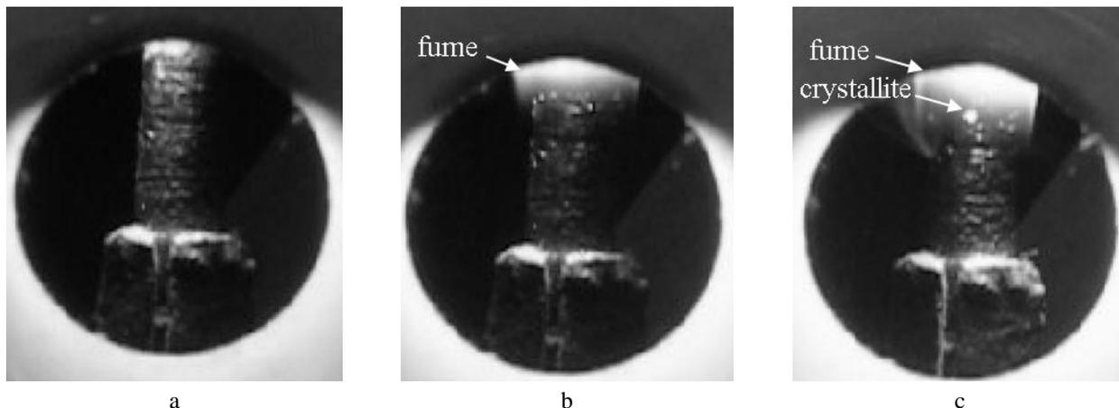
Fig. 5. View of anode at different process stages. Initial view - 7 s after arc ignition (a), appearance of white fume at 17 s (b), formation of  $\text{MoO}_3$  crystallites at 25 s (c)
