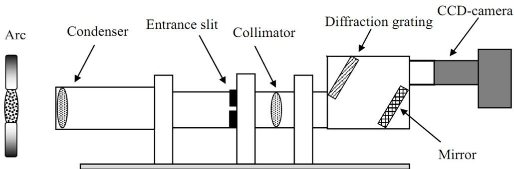
Fig. 2. Optical scheme of proposed experimental setup for emission spectroscopy
