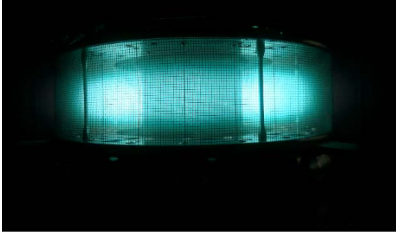
Fig. 6: wire-glow discharge, working parameters: p=1.5 Pa, I_D=81 mA and V_D=410 V.
