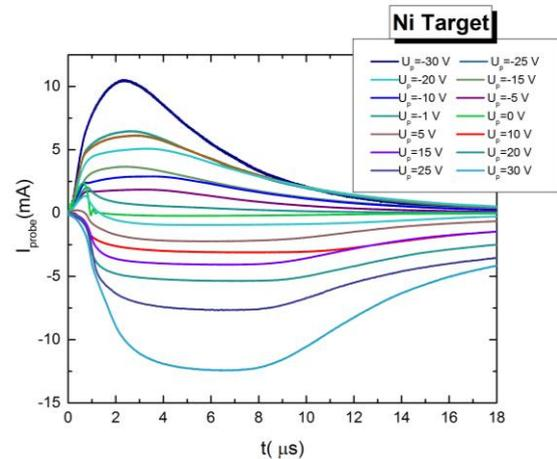
Figure 4. Transient ionic and electronic currents recorded by the Langmuir probe (placed at 6 mm, orthogonal on the plasma plume expansion direction) for different probe biases
