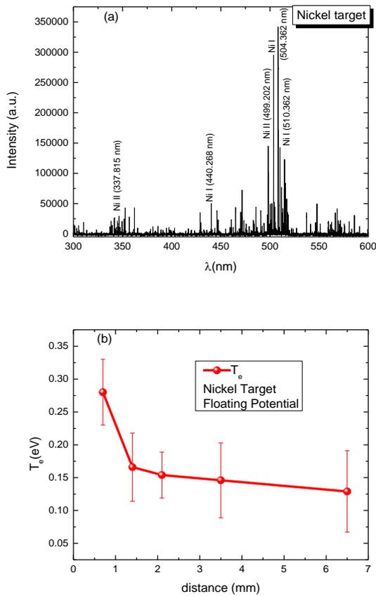
Figure 3. Emission Spectrum for a Ni laser produced plasma at 0.5 mm from the target (a) and the spatial evolution of the Nickel atoms excitation temperature (b).
