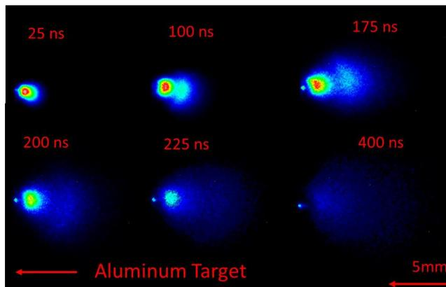
Figure 2. Temporal evolution of the Aluminum plasma plume emission recorded by the ICCD camera
