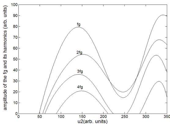
Fig.2 Resonance curves for the fundamental ghost frequency ( $f_g$ ) and its four harmonics
