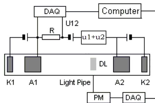
Fig.1 Sketch of the experimental set-up: K1, K2 – plane cathodes; A1, A2 – cylindrical anodes;  $u_1+u_2$  bi-harmonic perturbation; U12 – d.c. inter-anode biasing, DL – double layer structure, PM – photomultiplier, DAQ – data acquisition system
