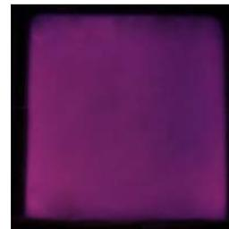
Fig. 1 The photo of RF-DBD along the radial direction (flow rate 2 slm, gap 3.3 mm, applied power 300 W and exposure time 1/100 s)
