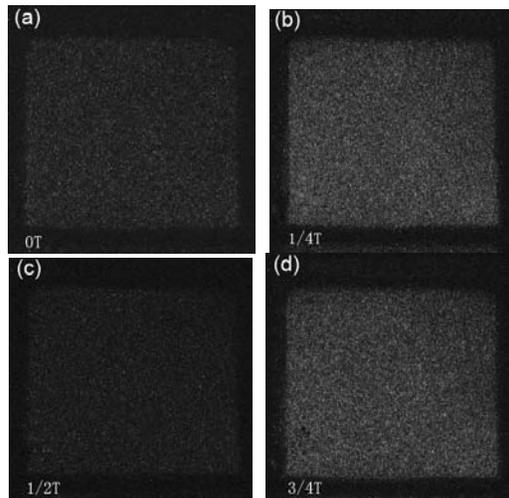
Fig. 2 The light emission images in radial direction during one cycle of RF taken at different periods with 2 ns exposure time and 200 cycles of accumulation by ICCD at  $t =$  (a) 0 T, (b) 1/4 T, (c) 1/2 T, (d) 3/4 T, respectively, where T is RF period
