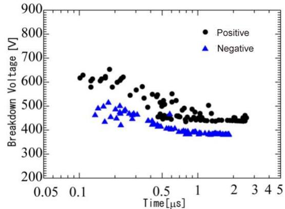
Figure 9.  $V-t$  characteristics across 3- $\mu\text{m}$  gap in 10-kPa air
