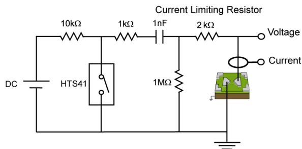
Figure 2. Measurement circuit
