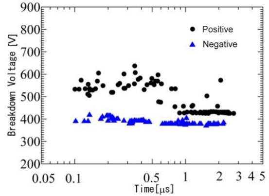
Figure 8.  $V-t$  characteristics across 10- $\mu\text{m}$  gap in 30-kPa air
