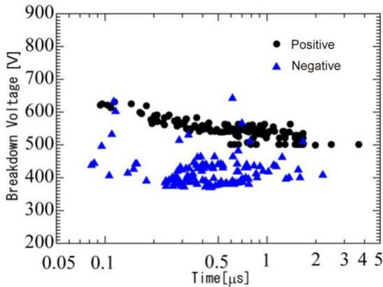
Figure 5.  $V-t$  characteristics across 30- $\mu\text{m}$  gap in 100-kPa air
