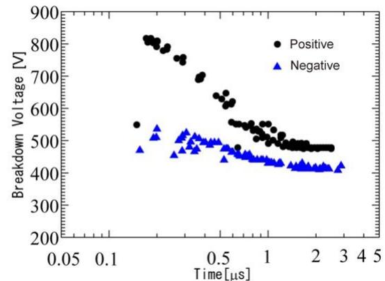
Figure 10.  $V-t$  characteristics across 3- $\mu\text{m}$  gap in 1-kPa air
