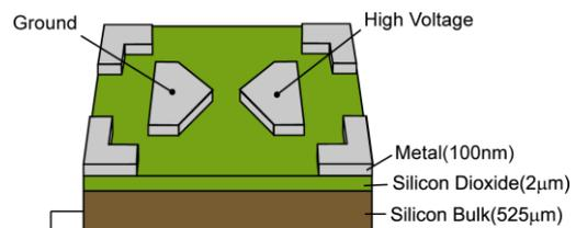
Figure 1. Micrometer-scale surface gap
