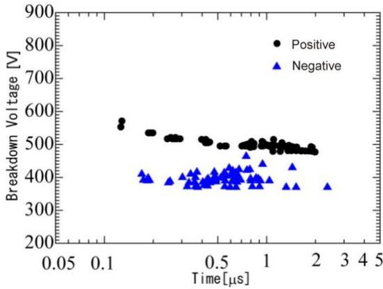
Figure 6.  $V-t$  characteristics across 10- $\mu\text{m}$  gap in 100-kPa air
