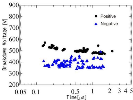
Figure 7.  $V-t$  characteristics across 3- $\mu\text{m}$  gap in 100-kPa air
