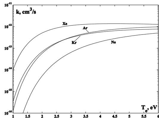
Fig.2 Excitation rate constant by electron impact
