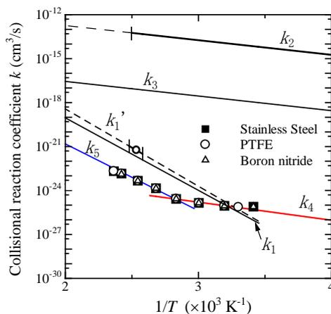
Fig. 5 Temperature dependence of reaction rate coefficients of ozone.
