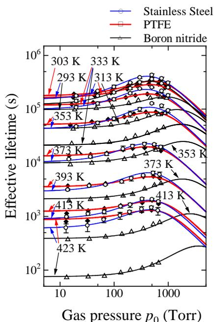
Fig. 3 Observed values of ozone effective lifetime against gas pressure. Black lines with circles: stainless steel, red lines with squares: PTFE, blue lines with triangles: boron nitride.
