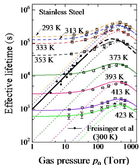
Fig. 2 Observed values of ozone effective lifetime against gas pressure. (Stainless steel)
