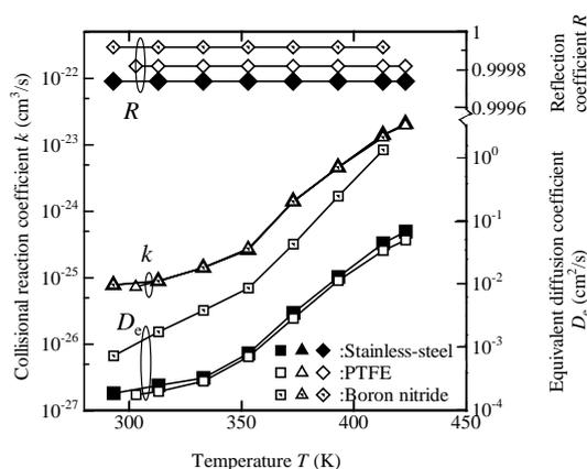
Fig. 4 Observed values of  $D_e$ ,  $R$  and  $k$  against temperature in three kinds of materials.
