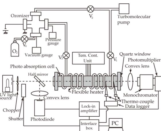
Fig. 1 Experimental apparatus. Ozone is formed in an ozonizer by corona discharge.
