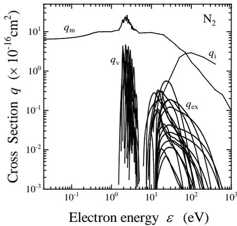
Fig. 4 Electron collision cross section of  $N_2$  [16].
