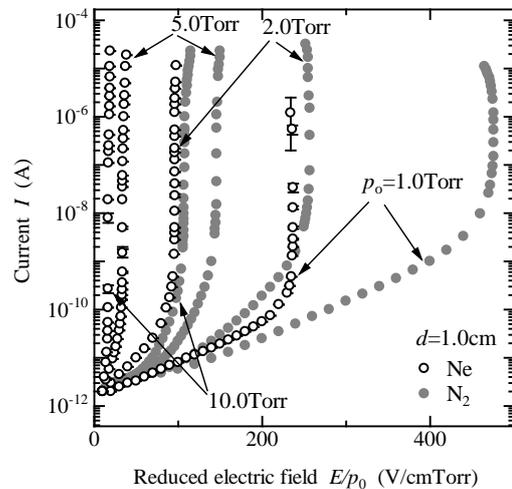
Fig. 3 Characteristic of current-voltage in Ne.
