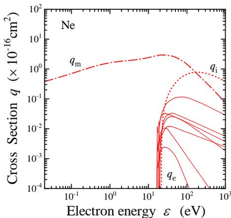
Fig. 5 Electron collision cross section of Ne [16].
