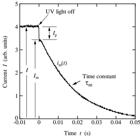
Fig. 2 Typical transient current waveform.
