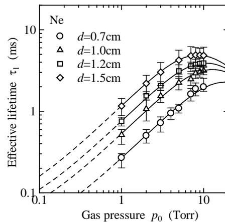
Fig. 7 Effective lifetime Ne metastable atoms in Ne.
