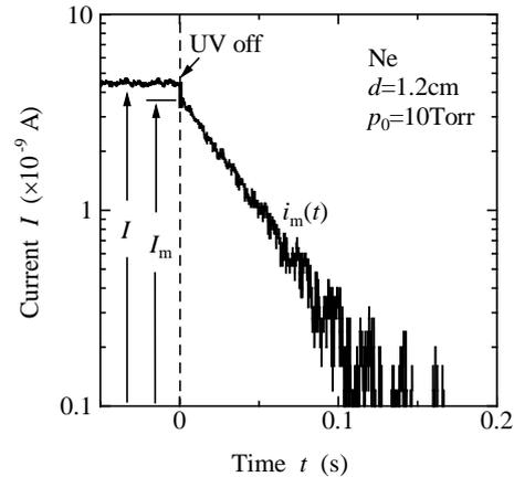
Fig. 6 Actual transient current waveforms at gas pressure of 10 Torr in Ne.
