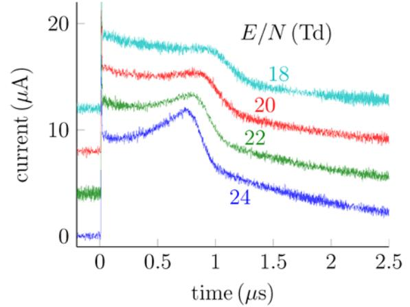
Figure 5: Measured current for 0.0305 % 2-C<sub>4</sub>F<sub>8</sub> in Ar, at the pressure of 100 mbar, electrode distance of 19 mm, and  $E/N$  between 18 and 24 Td. Offsets of +4  $\mu\text{A}$  have been added between measurements for better visibility.
