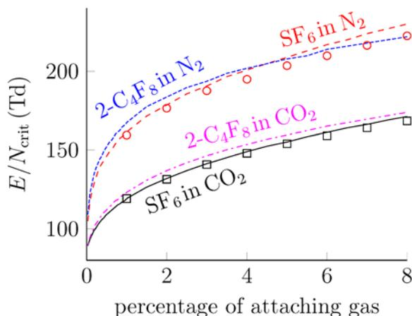
Figure 7:  $(E/N)_{\text{crit}}$  of SF<sub>6</sub> mixtures and 2-C<sub>4</sub>F<sub>8</sub> mixtures as a function of their percentage in the buffer gases N<sub>2</sub> or CO<sub>2</sub>. The lines are calculations using (1). The markers are simulations of SF<sub>6</sub> mixtures with N<sub>2</sub> or CO<sub>2</sub>, using the solver Bolsig+ with the complete cross section sets [6] for N<sub>2</sub>, [8] for CO<sub>2</sub> and [9] for SF<sub>6</sub>.
