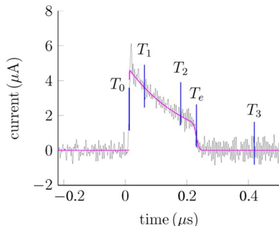
Figure 2: Current waveform in 0.0286 % of 2-C<sub>4</sub>F<sub>8</sub> in N<sub>2</sub> at a pressure 100 mbar,  $E/N$  of 60 Td and for an electrode gap distance of 15 mm.
