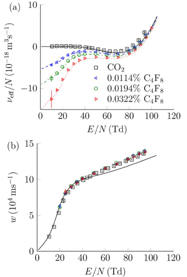
Figure 4: Swarm parameters in CO<sub>2</sub> and 2-C<sub>4</sub>F<sub>8</sub>/CO<sub>2</sub> mixtures at a pressure of 100 mbar and concentrations of 2-C<sub>4</sub>F<sub>8</sub> ranging from 0.011 to 0.032 %. (a) Effective ionization rate constant. (b) Electron drift velocity.
