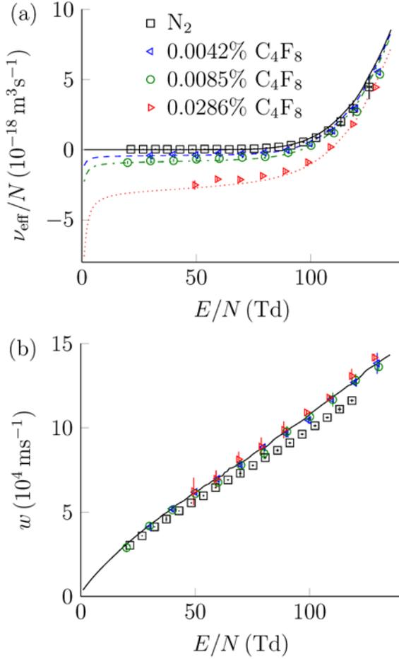
Figure 3: Swarm parameters in N<sub>2</sub> and 2-C<sub>4</sub>F<sub>8</sub>/N<sub>2</sub> mixtures at a pressure of 100 mbar and concentrations of 2-C<sub>4</sub>F<sub>8</sub> ranging from 0.004 to 0.0286 %. (a) Effective ionization rate constant. (b) Electron drift velocity.
