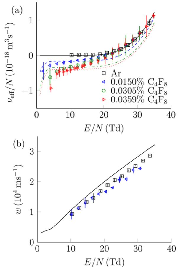
Figure 6: Swarm parameters in Ar and 2-C<sub>4</sub>F<sub>8</sub>/Ar mixtures at a pressure of 100 mbar and concentrations of 2-C<sub>4</sub>F<sub>8</sub> ranging from 0.015 to 0.036 %. (a) Effective ionization rate constant. (b) Electron drift velocity.
