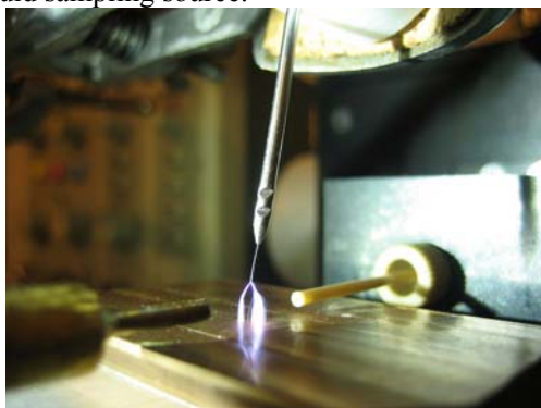
Figure 2. The discharge applied on aerosol jet used for liquid stream analysis.
