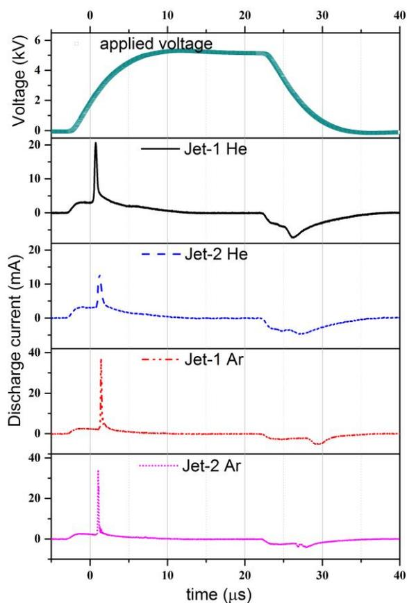
Figure 2. Typical waveforms of the applied voltage and discharge current for **Jet-1** and **Jet-2** in He and Ar.
