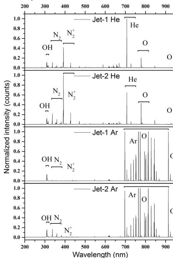
Figure 3. Emission spectrum for **Jet-1** and **Jet-2** plasma sources in He and Ar.
