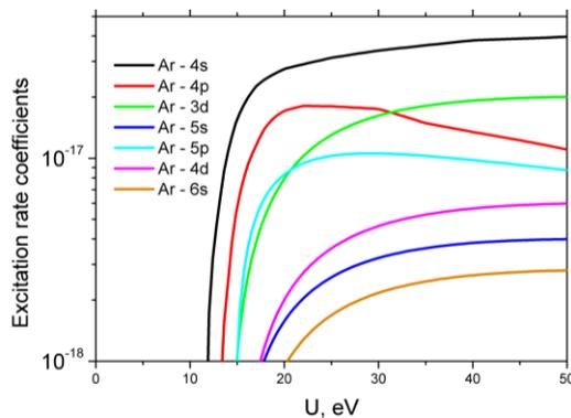
Fig. 3. Rate coefficients for direct excitation
