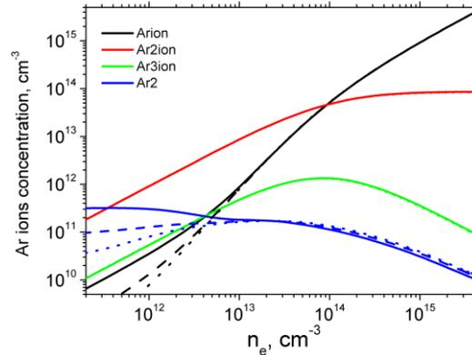
Fig. 8. Argon ions and Ar molecule concentration.
