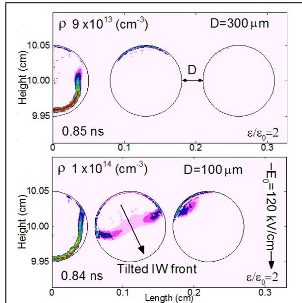
**Figure 7.** Tilted streamer front shown for the space charge density for the strings with two separations (300 and 100  $\mu\text{m}$ ). There is no streamer development in the middle bubble in the first case. For the smaller separation the tilted and planar front of the streamer in the middle bubble is clearly seen. Conditions: liquid with  $\epsilon/\epsilon_0 = 2$ ,  $E_0 = 120$  kV/cm.
