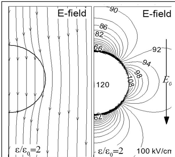
**Figure 2.** Initial distribution of the electric field (streamlines) and electric field (contours) around a 300  $\mu\text{m}$  bubble. The electric field is enhanced near the equator of the bubble and depleted near the poles. The streamlines show the direction of the electric field but not field magnitude. Conditions: the external medium is a dielectric liquid ( $\epsilon/\epsilon_0 = 2$ ), the applied external field  $E_0=110$  kV/cm.
