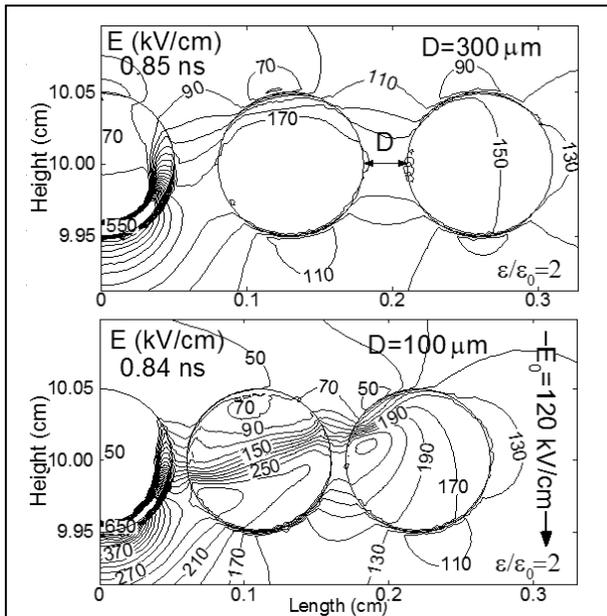
**Figure 6.** Electric field contours for the horizontal string of bubbles at  $t = 0.85$  ns. The distance between the bubble surfaces is 300 and 100  $\mu\text{m}$ . For large separation, there is no streamer development in the middle and the right bubbles. For smaller separation, the tilted electric field vectors result from the superposition of the applied field and the field from the space charge of the streamer. Conditions: liquid with  $\epsilon/\epsilon_0 = 2$ ,  $E_0 = 120$  kV/cm.
