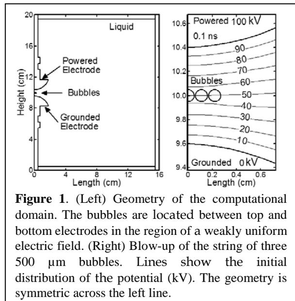
**Figure 1.** (Left) Geometry of the computational domain. The bubbles are located between top and bottom electrodes in the region of a weakly uniform electric field. (Right) Blow-up of the string of three 500  $\mu\text{m}$  bubbles. Lines show the initial distribution of the potential (kV). The geometry is symmetric across the left line.
