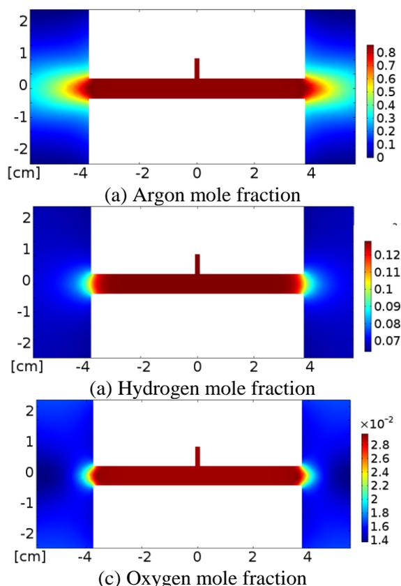
**Figure 2:** Mole fractions of the background gases plotted in a horizontal cross-section through the discharge chamber for  $Q_{\text{Ar}} = 145 \text{ sccm}$ ,  $Q_{\text{H}_2} = 22 \text{ sccm}$  and  $Q_{\text{O}_2} = 5 \text{ sccm}$ .
