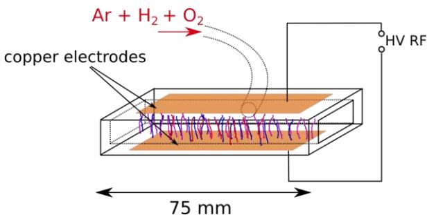
**Figure 1:** A schematic view of the dielectric barrier discharge. The setup is opened to ambient atmosphere on the sides.
