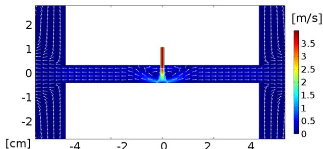
**Figure 3:** Gas velocity magnitude and direction plotted in a horizontal cross-section through the discharge chamber for  $Q_{\text{Ar}} = 145 \text{ sccm}$ ,  $Q_{\text{H}_2} = 22 \text{ sccm}$  and  $Q_{\text{O}_2} = 5 \text{ sccm}$ .
