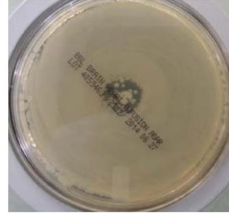
**Figure 2:** E. coli inactivation area (dark) for the jet-helium distance of 1.5 cm and helium flow rate of 5.5 slm in a Petri dish with 10 cm diameter.
