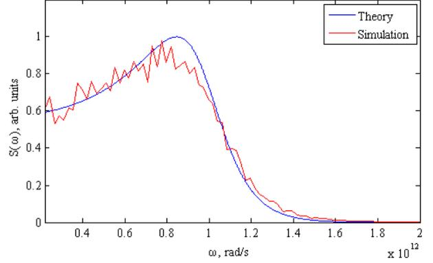
Fig.1 Spectrum of electron density fluctuations  $S(k, \omega)$  for  $k = 3.14 \cdot 10^4 \text{ m}^{-1}$  and plasma parameters as specified in Sec.3.
