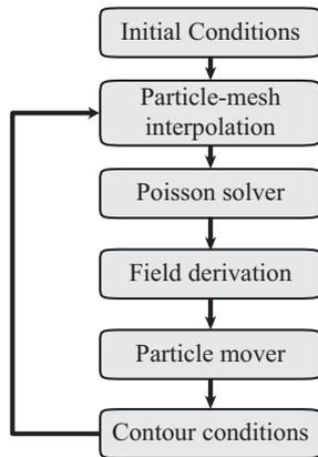
**Figure 2.** Flow chart of the code of the simulations
