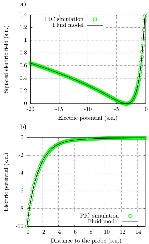
**Figure 3.** Comparison between results provided by the simulations and fluid models using the units of the simulation (s.u.): a) planar probe and b) cylindrical probe.
