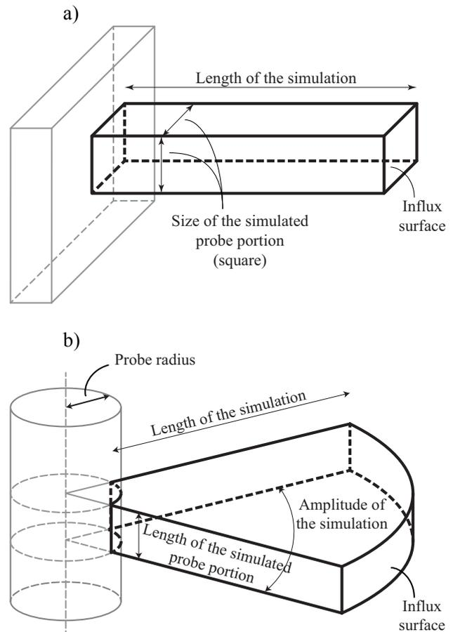
**Figure 1.** Simulation domain for both geometries: a) infinite planar probe and b) infinite cylindrical probe.
