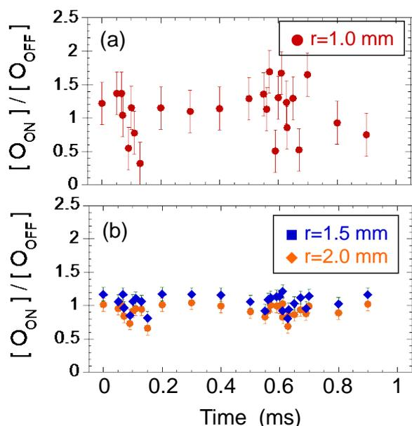
Fig. 3 Temporal variations of the densities of atomic oxygen observed at a radial position of (a) 1.0 mm and (b) 1.5 and 2.0 mm.
