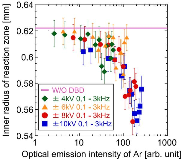
Fig. 1 Relationship between the radius of the reaction zone and the optical emission intensity of Ar.
