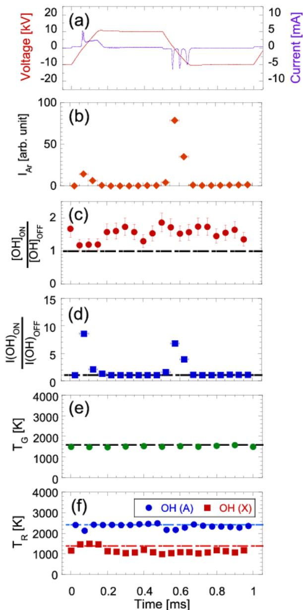
Fig. 2 Temporal variations in various quantities in a cycle of DBD: (a) waveforms of the discharge voltage and discharge current, (b) optical emission intensity of Ar, (c) density of OH( $X^2\Pi$ ), (d) optical emission intensity of OH, (e) gas temperature, and (f) rotational temperatures of OH( $X^2\Pi$ ) and OH( $A^2\Sigma^+$ ).
