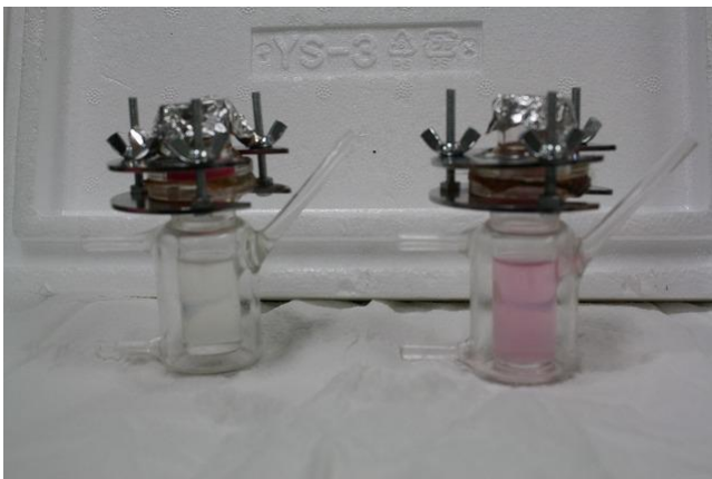
Fig. 5 Photograph of the Franz-type diffusion cell for the transepidermal absorption test using phenol red (left: control sample, right: after 5 min. microplasma irradiation).
