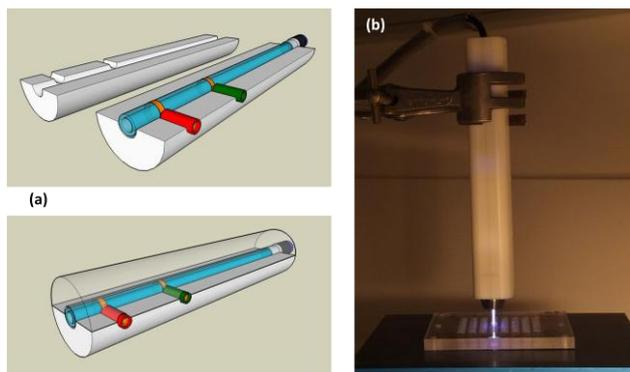
**Figure 1(a)** Schematic diagram of the kHz-driven plasma source used in this study and **(1b)** Photograph of hand held non-thermal plasma source used in the present study.
