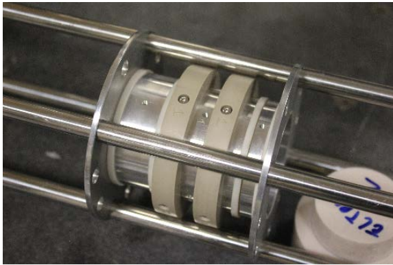
Fig. 4: Picture of a part of the electrode stack, showing an azimuthally split electrode, made out of four sectors with a 90 degree angular span mounted on two PEEK rings.
